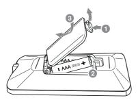
Remove the battery cover on the rear of the remote control, and insert the batteries with  $\oplus$  and  $\oplus$  matched correctly.
