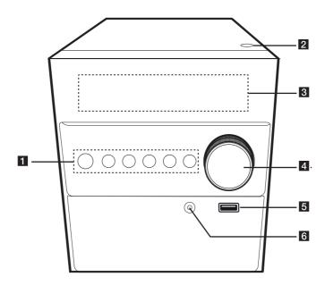
1 U/l (Standby/On) Switches the unit ON or OFF.
