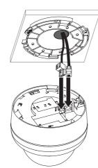
4. Assemble the camera and mounting bracket after align the front part of the camera and mounting bracket. Connect the unit by following step 1 and 2.
