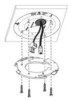
3. Connect the cables to the cable jacks of the camera body.
