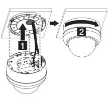
Be careful of sharp edge after removing the cap of cable conduit.
