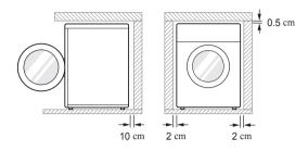
**Level floor :** Allowable slope under the entire washing machine is 1°.
