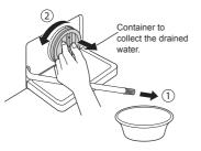
4 After cleaning, turn the pump filter and insert the drain plug.
