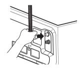
3 Adjust the hose clip in place to prevent leaking.
