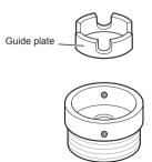
3 Push the adapter onto the end of the tap so that the rubber seal forms a watertight connection. Tighten the four fixing screws and the adapter ring plate.
