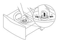
2 Open the cap and remove lint and then wash out.
