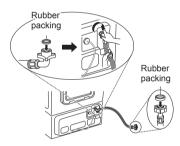
3 Connect the additionally provided water supply hose of the front-loading washing machine to the water supply hose connector and water faucet.
