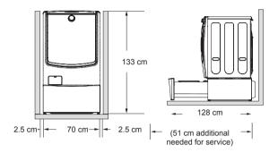
**Level floor** : Allowable slope under the entire appliance is 1°.
