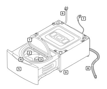
**1** Door 2 Drum **3** Lint Filter 4 Control Panel **[5]** Drawer 6 Water Supply Hose 7 Power Plug Water Drain Hose 8 ൭ Leveling Feet
