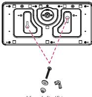
2-Screws for Stand Fixing, 2-Washers for Stand Fixing, 2-Nuts for Stand Fixing (Supplied with TV)
