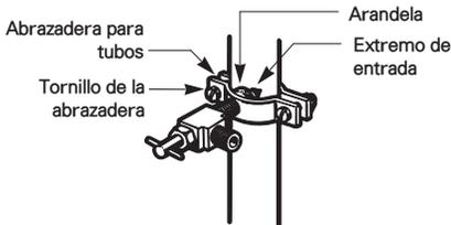
6 ENCAMINE LA TUBERÍA.
