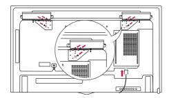
3 Then connect the speaker cable. After installing your speakers, use holders and cable ties to organize the speaker cables.
