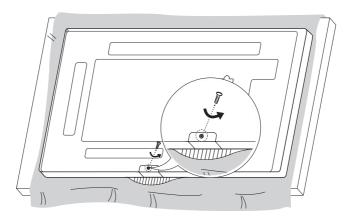
2 After removing the screw, remove the LG Logo Bracket. Attach the LG Logo Bracket with a screw, aligning it with the hole on the right side.
