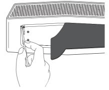
In case that the unit freezes due to malfunction, remove the rubber sleeve and press the reset hole using an object like a thin pin. Then the unit is turned off completely.
