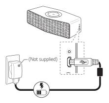
If the battery is fully charged in charging mode, indicator is changed from red to green.
