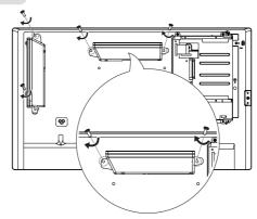
3 Then connect the speaker cable. After installing your speakers, use holders and cable ties to organize the speaker cables.
