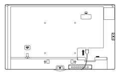
2 Mount the speakers by using screws as shown below. Make sure the power cable is disconnected before making a connection.
