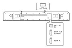
USB port · · · · · Connect to a USB device. OPTICAL IN ..... Connect to an optical device. HDMI OUT (TV ARC)····· Connect to a TV. HDMI IN .....Connect to device with HDMI OUT.
