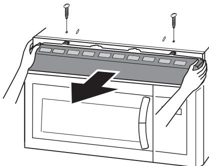
**7** Slide the bottom of the vent grille into place. Push the top in until it snaps into place. Insert and tighten the vent grille mounting screws.
