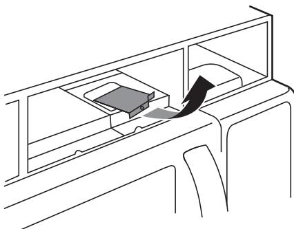
**5** Replace bulb with a 30 watt appliance bulb.
