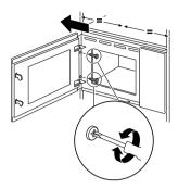
4 Check the clearance to the adjacent appliances. The clearance to the adjacent appliances must beat least 5 mm.
