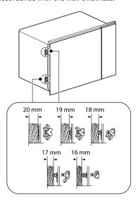
2 Insert the appliance into the unit and move it to the right.
