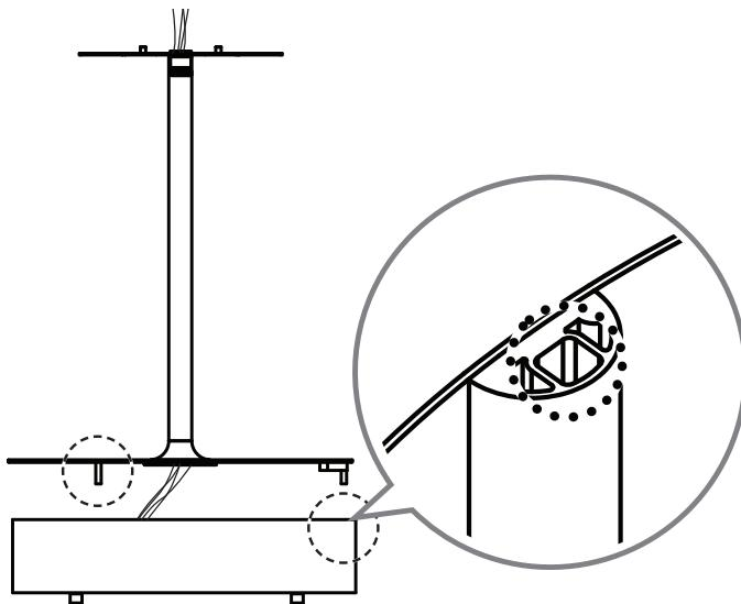
15 Identify the Front and Rear HDMI cables and 16/22 pin cables, then pick up the set and attach it to the frame.
