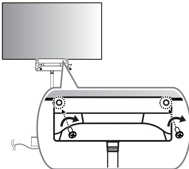
21 Fasten 6 screws (M4 x L8) to the bottom part of the T-con cover.
