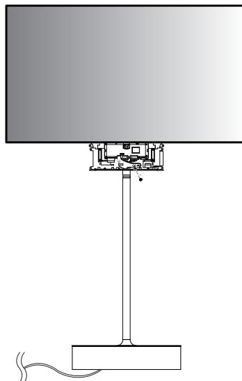
16 Connect the HDMI cable with the label marked 'FRONT' to the front side. Insert the 16/22 pin cable without the red mark into the cable holder and attach it using a screw (M3 x L4.5).
