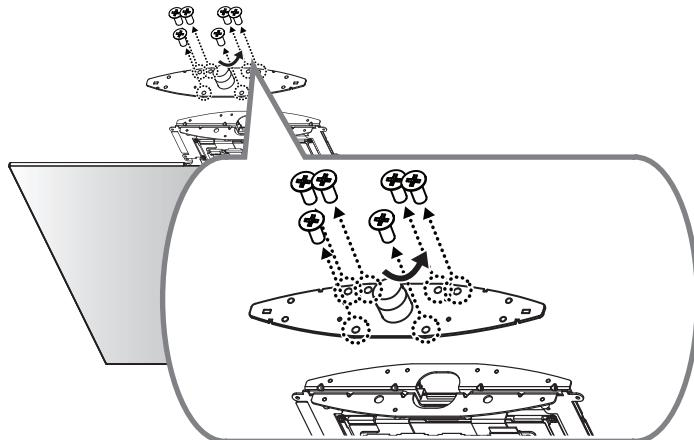
4 Affix the pipe to the Cylinder Stand Top and the Top body to the pipe. Hold the pipe and pull up to open the Cylinder Stand Top.
