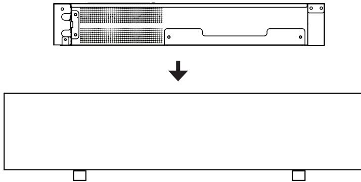
12 Pass the power cable through the hole in the bottom near the stand connector and into the inside of the stand, and then attach the cable to the Signage box.
