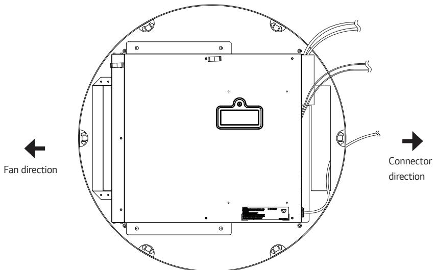
13 Install the Signage box with the attached cables onto the stand base and attach it using four screws (M3 x L4.5).
