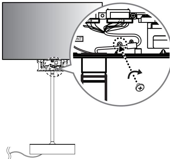
17 Connect the HDMI cable without the label marked 'FRONT' to the rear side. Insert the 16/22 pin cable with the red mark into the cable holder and attach it using a screw (M3 x L4.5).
