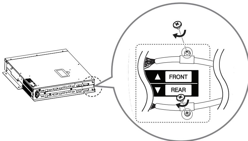
10 Position the jack cover to fit the cables to the cut spaces and then attach it using the 2 screws (M3 x L4.5).
