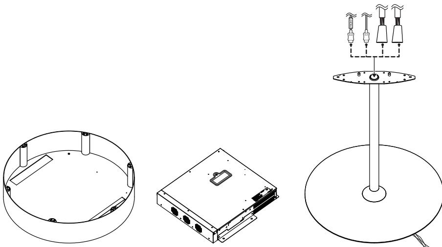
8 Connect the cables passed through the pipe to the Signage box. The Front cable must be connected to the upper part and the Rear cable must be connected to the lower part. The 16/22 pin cable with the red mark must be connected to the upper part.
