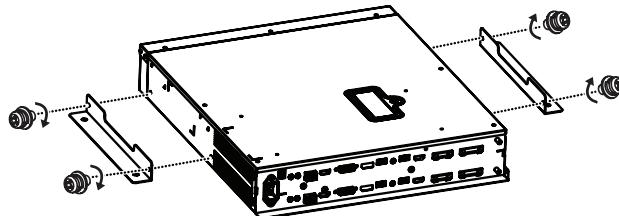
3 Loosen the six screws and remove the frame from the set.
