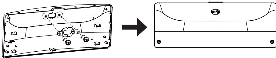
19 Cover the front side with the side of the T-con box cover that has the IR receiver and attach it using four screws ( $\Phi 3 \times L6$ ) on the opposite side.
