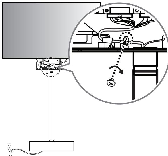
18 Remove the two screws, change the direction of the LG logo, and then reassemble.
