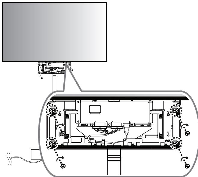
20 Cover the rear side with the other T-con box cover and attach it using 2 screws ( $\Phi 3 \times L10$ ).
