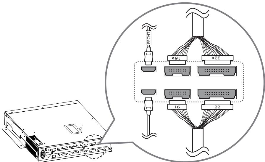
9 Attach the 16/22 pin cables using the 2 screws (M3 x L4.5).
