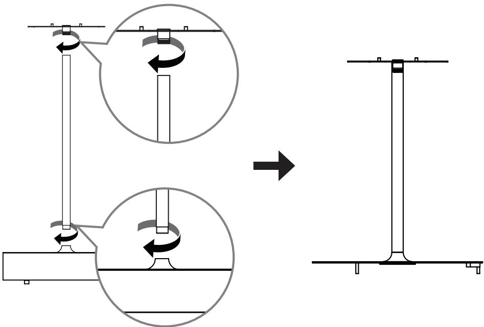
5 Attach the pipe to the frame by fastening a screw (M3 x L5.5) in the screw hole on the top of the pipe.
