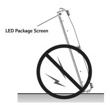
2 If the product is tilted towards the edge of the LED package screen, the bottom (corner) of the product may be damaged.
