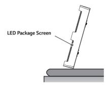
3 Place the product with the LED package screen facing down. To protect the screen, lay the protective pad in the box on the floor.
