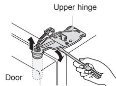
7 Remove the freezer and fridge compartment door by lifting it upward. At this time, the door should be lifted enough for the steel pipe to be completely pulled out.
