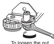
2 Adjust the difference in the height of the appliance door by rotating the adjustment hinge pin clockwise or counterclockwise with an 8 mm spanner.
