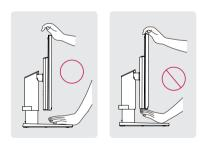
Be careful not to touch or press the screen area when adjusting the angle of the monitor.
