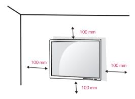
To install the monitor to a wall, attach a wall mounting bracket (optional) to the back of the monitor.
