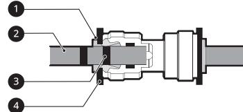
① Collet ② Water supply line ③ Insert line ④ Clip
