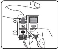
Connect the black stripe of each wire to the terminals marked - (minus) and the other end to the terminals marked + (plus).
