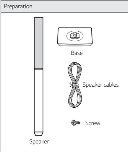
1. Attach the pole to the base, then secure the connection with a supplied screw.
