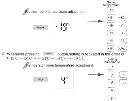
How to adjust the temperature in the refrigerator compartment
