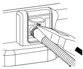
3 Screw in the band to secure the drain hose of the dryer onto the stacking bracket.
