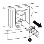
Connect the drain hose of the dryer and secure the hose clamp.
