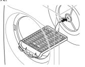
Place the dryer rack on the structure above the lint filter and press it to complete assembly.
