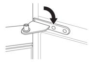
5 Tighten the two hinge bolts.
