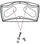
2-Screws for Stand Fixing, 2-Washers for Stand Fixing,
