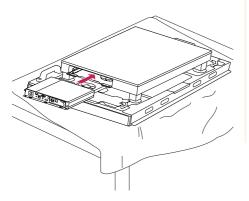
Secure the MP700 to the product using the two screws provided.
