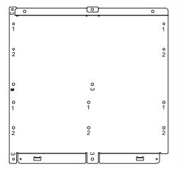
Attach the guide bracket to the back of your monitor. (3 or 4 screws are required depending on the model.)
