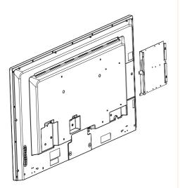
Assemble to the guide bracket with the fixing screws.
