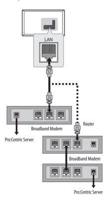
① Connect the **LAN** port of the Modem or Router to the **LAN** port on the TV.
