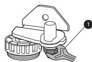
3 Use the spanner ① to fasten the keeper nut by turning it to the right.
