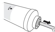
3 Push the pipe into the water filter, making sure the end is fully sealed.
