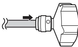
**2** Ensure that the rubber washer is fitted to the inside of the tap connector before screwing it onto the tap.
