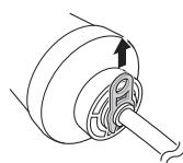
2 Pull the pipe out from the water filter.
