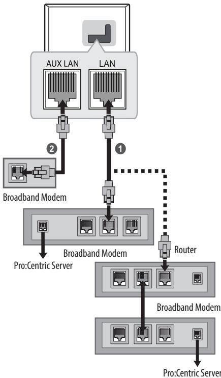
① Connect the **LAN** port of the Modem or Router to the **LAN** port on the TV.
