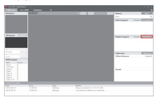
2 To implement X-ray shot. Calibration SW will wait for a X-Ray acknowledgement signal from DXD and it will display a waiting sign.
