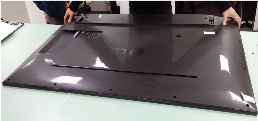
(1) Disassemble Screw and then Hold B/C Bottom Side.
