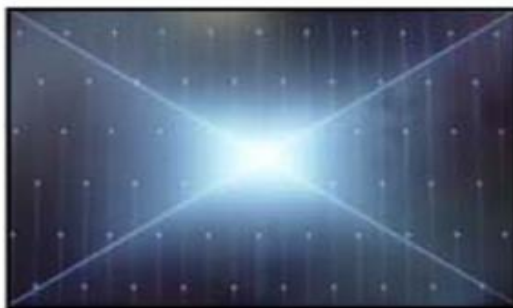
Solder defect, Short/Crack
