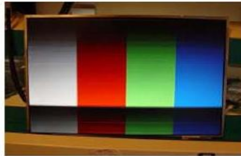
Horizontal Block Gate TAB IC Defect
