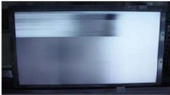
Horizontal Block Gate TAB IC Defect
