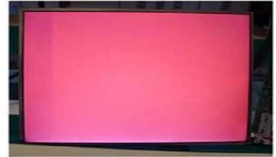
Vertical Block Source TAB IC Defect
