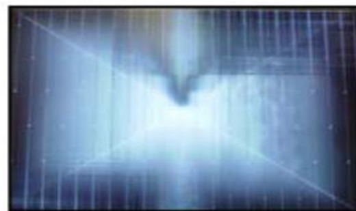
Solder defect, Short/Crack
