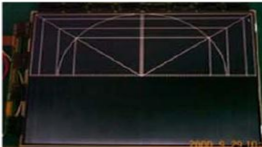
Horizontal Block Gate TAB IC Defect
