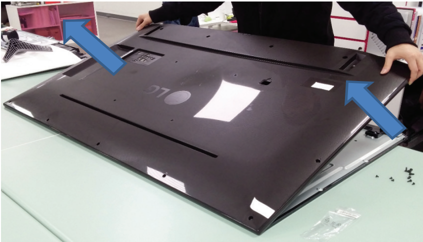
(2) Pull the upward at point of picture.
