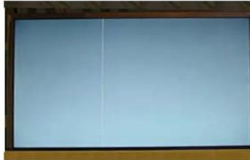
Vertical Line Source TAB IC Defect
