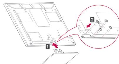
Make sure to assemble the front and rear side of the stand.
