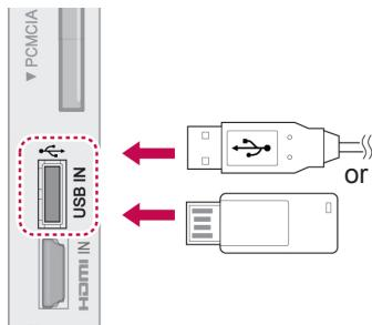
To disconnect a USB storage device, make sure to end the connection properly to prevent damages to the TV or files.
