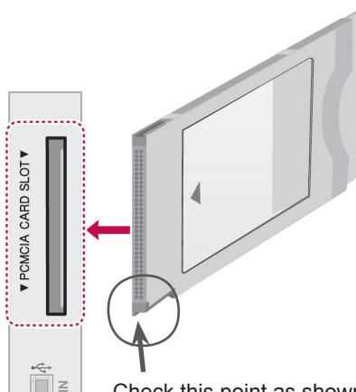
Check this point as shown and insert the CI Module.
