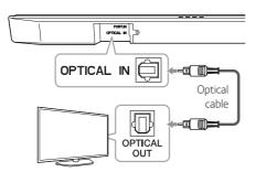
2. Set up the sound output of TV to listen to the sound through this unit: TV setting menu → [Sound] → [TV Sound
