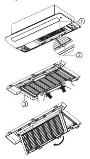
3. As shown in the figure, pull on the handle and remove the deodorization filter.
