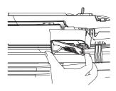
5. Use a slightly wet cotton swab to wipe dust off the lens, and then use a dry swab to remove the moisture.
