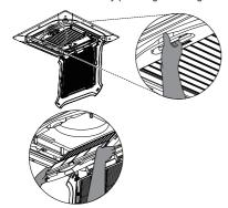
3. Remove the photocatalyst Deodorization filter by pulling upward.
