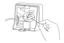
Tighten the rubber cap, close the PM1.0 sensor case, and assemble the PM1.0 Sensor corner cover to its original position.
