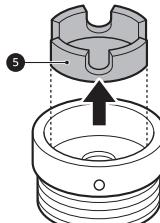
3 Push the adapter onto the end of the tap so that the rubber seal is connected to be watertight. Tighten the 4 fixing screws and the adapter ring plate.
