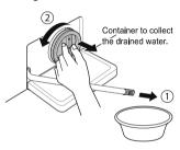
3 Remove any extraneous matter from the pump filter.
