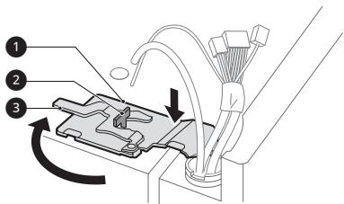
3 Connect all the wire harnesses and the ground screw.
