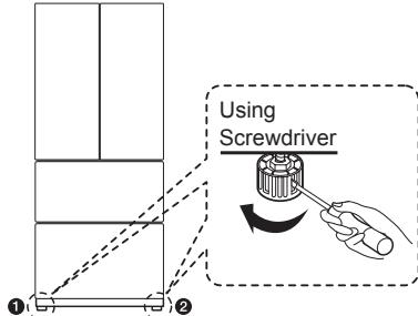
To level the refrigerator, use a screwdriver to turn the leveling feet until they are in firm contact with the floor. The front of the refrigerator can be slightly higher than the rear to make shutting the doors easier.
