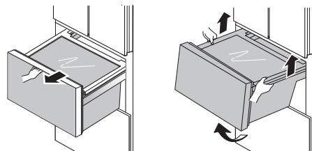
To reassemble the drawer, align it with the rails and insert it until it stops, lift it to clear the safety rail stops and push it in completely.
