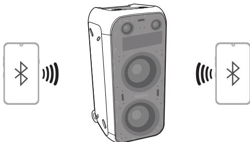
4 When two smartphones and the product are connected, the BT LED turns on.
