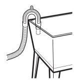
3 Use the provided tie strap to secure the drain hose in place.
