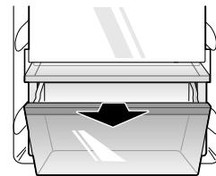
**3** Lift the drawer up and remove it by pulling it out.
