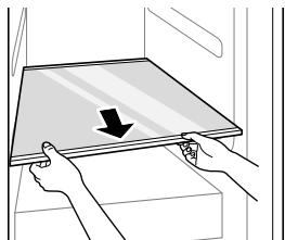
2 Tilt the shelf slightly and remove it by pulling it out.
