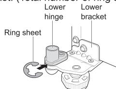
3 Resecure the bracket screw after fitting the ring sheets before refitting the door. When the door is refitted, steps 1,2 and 3 of adjusting the height of the door can then be repeated.
