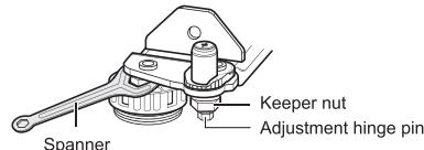
**1** Loosen the keeper nut by rotating it counterclockwise using a 19 mm spanner.
