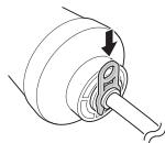
3 Repeat on the other end of the filter using the remainder of the water tube.
