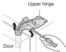
**7** Remove the freezer and fridge compartment door by lifting it upward. At this time, the door should be lifted enough for the steel pipe to be completely pulled out.
