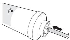
2 After inserting the tube securely into the filter, fit the locking clip into position under the pull up collar.
