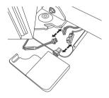
3 Remove the two hinge bolts.
