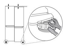
Open both doors and check to make sure that they close easily. If the doors do not close easily, tilt the refrigerator slightly more to the rear by turning both levelling legs to the left. It may take several more turns, and be sure to turn both levelling legs the same amount.
