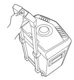
3. Release the lock button to lock the handle in place.
