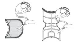
${f 3}$  If the lint filter has become very dirty or clogged with fabric softener, wash the lint filter in warm, soapy water and allow it to dry thoroughly before reinstalling.
