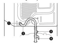
● 3/8"→ 5/16" NPT Gas Connection (from dryer to hose - gas tank)
