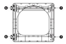
With the hinges and cover caps in the new locations, remount the inner door frame onto the outer door frame with the screws removed in step 3 above.
