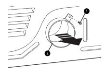
Press the tabs on the knockout and carefully remove the knockout for the desired vent opening. (Right-side venting is not available on gas models.) Press the adapter duct onto the blower housing and secure to the base of the appliance as shown.
