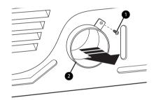
Press the adapter duct 3 onto the blower housing and secure it to the base of the appliance as shown.
