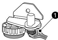
2 Use the spanner ② to adjust the height by turning the adjustment hinge pin to the left or to the right.
