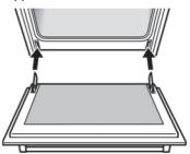
Position the door so that the hinge grooves engage on both sides.
