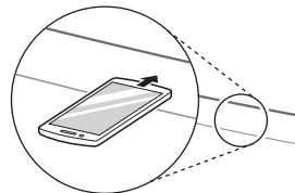
**2** Press and hold the **Ambient** and **Cont.** buttons for 3 seconds or longer while holding your phone to the speaker until the data transfer is complete.
