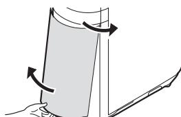
**3** Lift up the tip of the filter and turn it counterclockwise to remove it.
