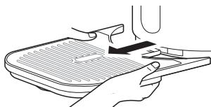
**2** Turn the water tap sideways and hold the lower part of the filter cover and pull it forward.
