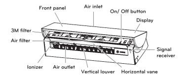
\* The feature can be changed according to a type of model.
