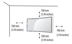
To install the monitor to a wall, attach a wall mounting bracket (optional) to the back of the monitor. Make sure that the wall mounting bracket is securely fixed to the monitor and to the wall.
