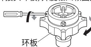
**2 如果水龙头过大而与接头不匹配，请拆下导向板。**
