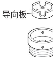
**3 将接头往上推至水龙头末端，从而使橡胶密封圈形成水密连接。拧紧四颗固定螺丝和接头环板。**
