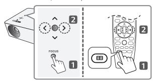
**3** If the angle of the projection is not perpendicular, use the [Keystone] function.
