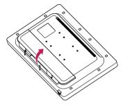
Remove the cable holder screws tightened on the back of the monitor. After installing the cables, tidy them up using the cable holders. Once the cables are tidy up, assemble it using the cable holder screws.
